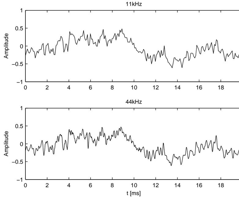
Figure 3.2: The effects of down-sampling on a 20ms sequence of *Freak on a Leash*. This sequence is the same as the one in the last subplot of Figure 3.1(a).
