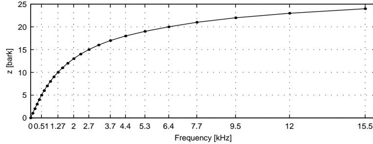
Figure 3.4: The basic characteristics of the critical-band rate scale. Two adjoining markers on the plotted line indicate the upper and lower frequency borders for a critical-band. For example, the 24th band starts at 12kHz and ends at 15.5kHz.
