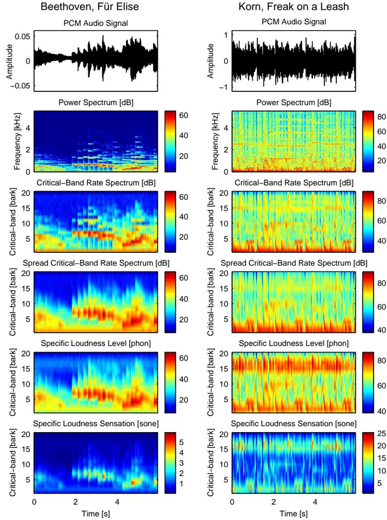
Figure 3.7: The feature extraction steps from the 11kHz PCM audio signal to the specific loudness per critical-band.
