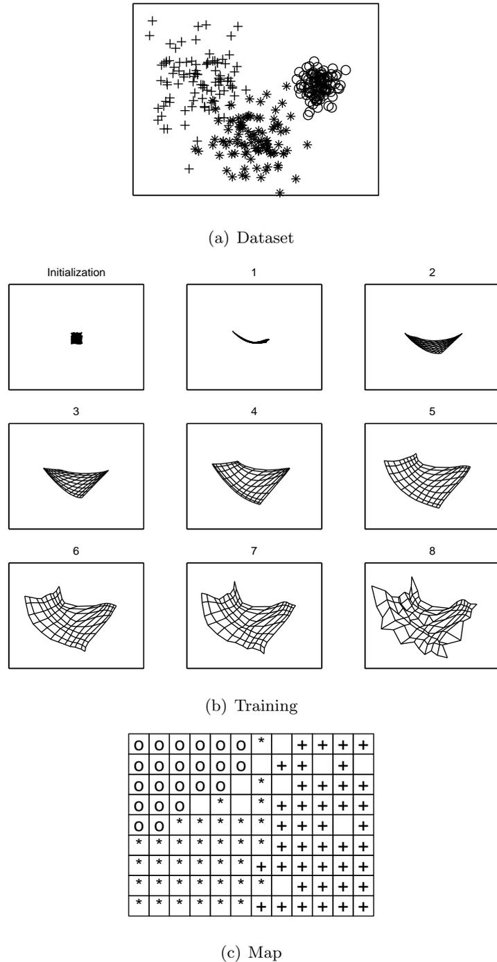
Figure 4.1: The batch SOM algorithm illustrated with a simple 2-dimensional toy dataset. Starting with a random initialization 8 training iterations are calculated and the position of the model vectors in the data space visualized. Finally the units are labeled with the most frequent class they represent.
