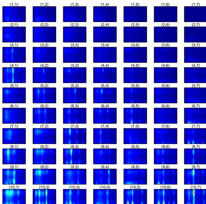
Figure 4.5: The model vectors of the SOM in Figure 4.3. Unlike Figure 4.4 the color coding is not scaled to each model vector instead it is scaled to the all model vectors. Thus the color coding corresponds to the way the SOM algorithm sees the model vectors.
