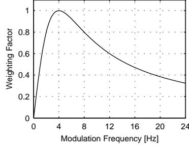
Figure 3.9: The relationship between fluctuation strength and the modulation frequency.
