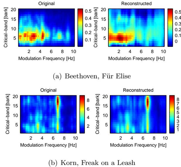
Figure 4.7: Comparison between the 1200-dimensional data space and the 80-dimensional eigenspace. The same as in Figure 4.6, except that the images are reconstructed from the 80-dimensional eigenspace instead of the 20-dimensional eigenspace.
